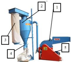
Fig. 1. Hammer mill MC 22: 1 – hammer mill; 2 – exhauster; 3 – cyclone with support and dust collector bag; 4 – grinding material evacuation vent; 5 – electric motor
